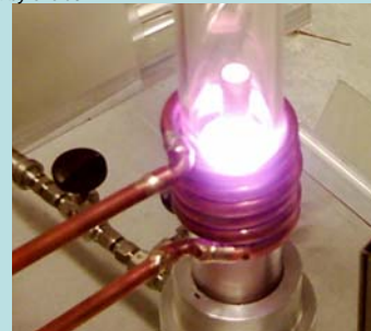
Fig 2. Radio frequency furnace used for the synthesis .
