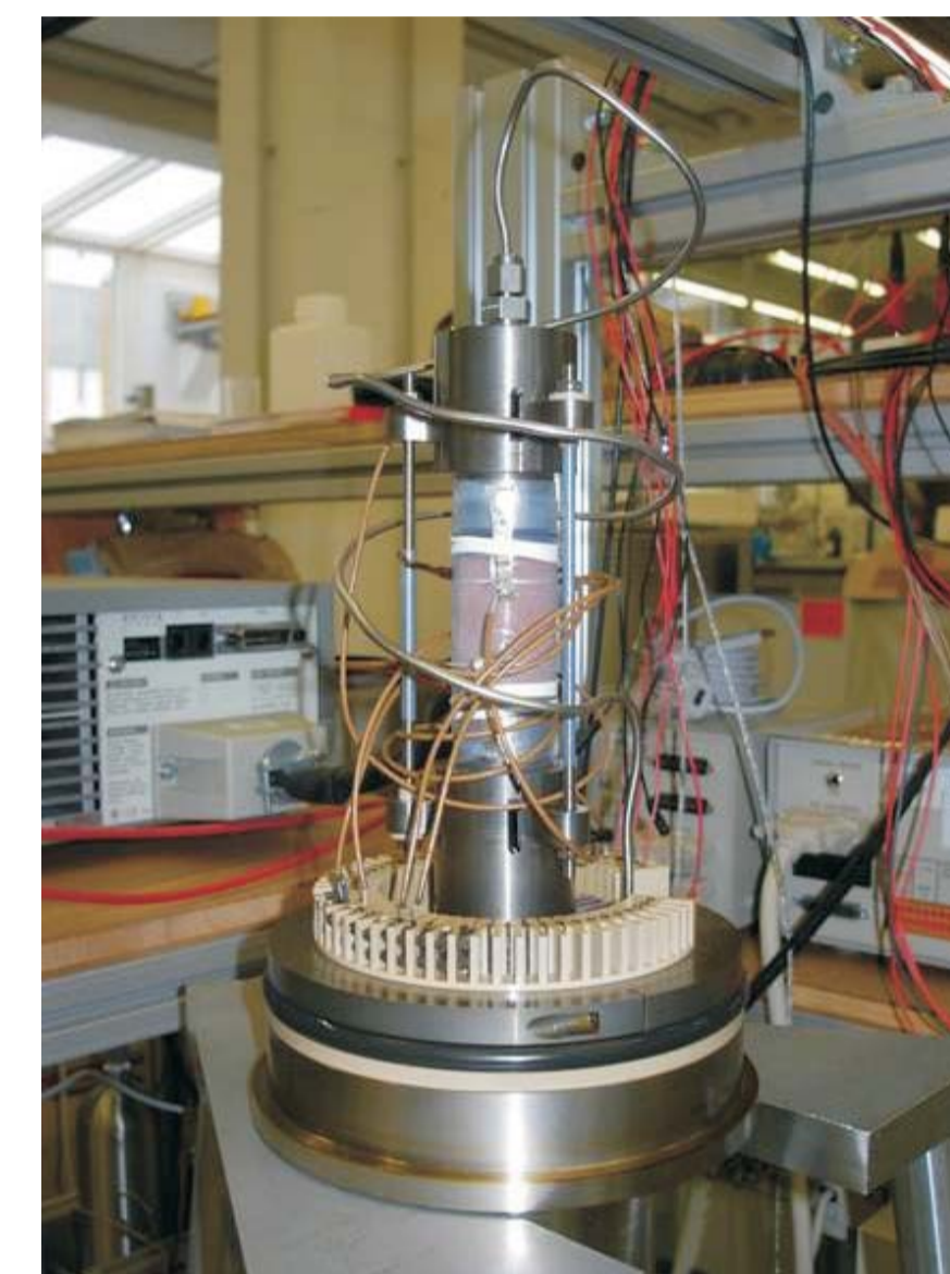
Fig. 3: Detail of the mounted specimen assembly. A Rotliegend rock-sample is located in the centre. Fluid is fed through the capillary system (silvery-gray spiral). Temperature and conductivity sensors are visible (brown cables).
