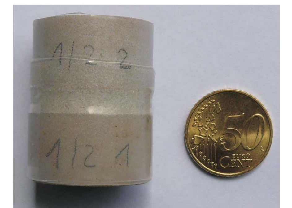
Fig. 4: Photograph of a flow-through sample consisting of two Fontainebleau quartz-sandstone discs with a sand pack in the centre. The sand consists of quartz and labradorite (plagioclase feldspar).
