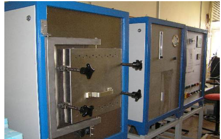
Gas controlled Linn™ Furnace Powder metallurgy lab., Department of Metallurgical and Materials Engineering, I.T.U
