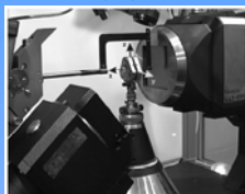
Figure 3. The diamond anvil cell mounted on the diffractometer with indicated x, y and z directions.
