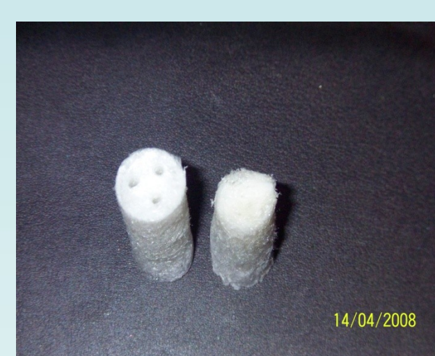
Figure 1: scaffold with and without channels.
